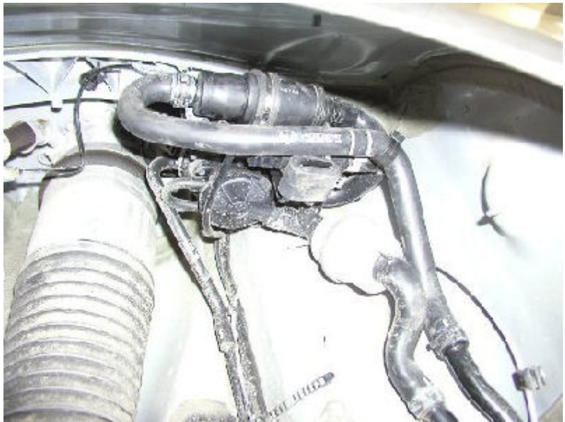
Figure 3. Filter location in left-rear wheel well on an affected A8 vehicle.
