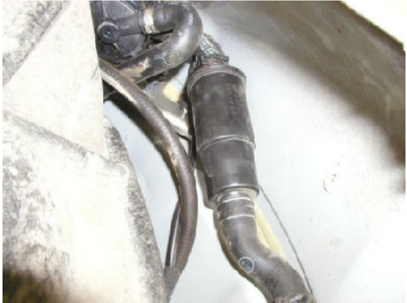
Figure 2. Filter location in left-rear wheel well on an affected A6 vehicle.
