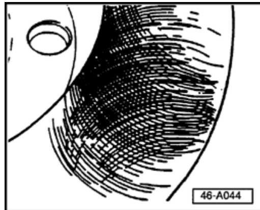
Figure 2. Lightly sand the brake disc.
