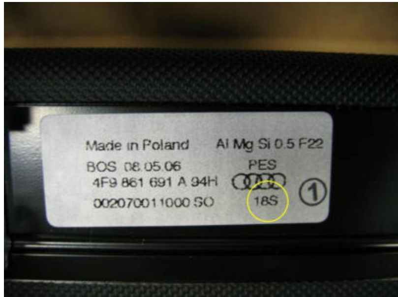
Figure 1. You will find a white sticker similar to this on the net partition. In this figure, the parts version is circled in yellow.
