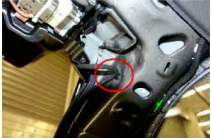
Figure 5. A reinforcing hose must be installed in the area marked in red to protect the rear window washer hose.
