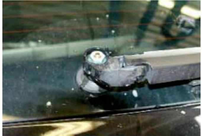
Figure 8. Pull cap off rear window washer nozzle.
