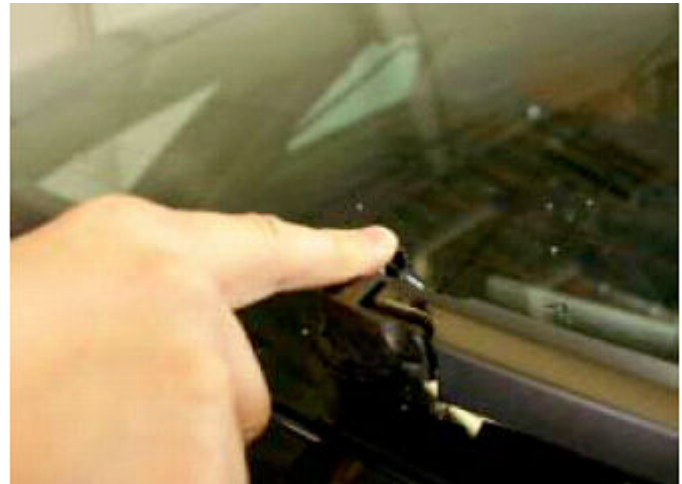
Figure 9. Have a second mechanic hold a finger over the washer nozzle to keep it closed. Operate the rear window washer for approximately five seconds.
