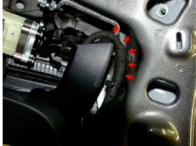
Figure 14. Ensure the hose has sufficient clearance and does not chafe when the tailgate is closed.
