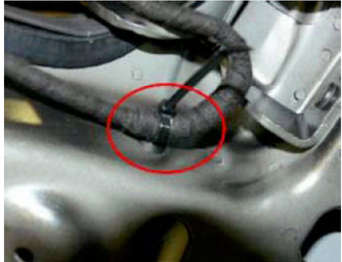
Figure 12. Secure the hose with a cable tie at this spot.
