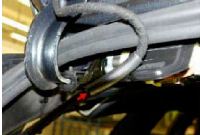
Figure 10. The lower end of the reinforcing hose starts at the point marked here with an arrow.
