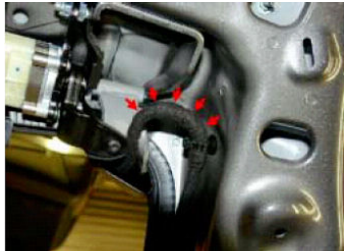
Figure 13. Ensure the hose has sufficient clearance and does not chafe when the tailgate is open.
