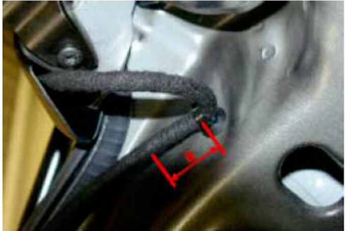
Figure 6. Measure a distance of 15 mm (A) from the cable tie.
