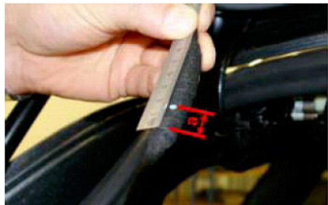
Figure 11. Mark 15 mm from the end of the reinforcing hose.
