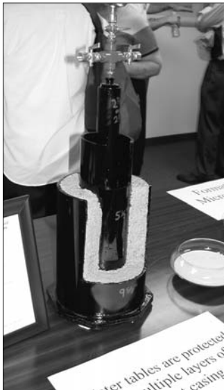
Texas-based Chief Oil and Gas drilled the first Marcellus Shale well in Lycoming County. In the left photo the company displays steel and cement casing used to protect groundwater from drilling fluids. The above photo is a compressor station built by the company.
